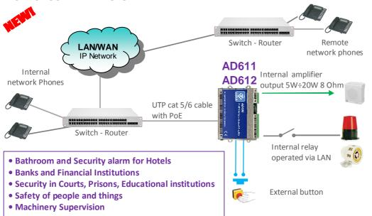
By connecting a button or an external contact, AD611-612 can call a phone number programmed to alert the event with a warning specific message.
